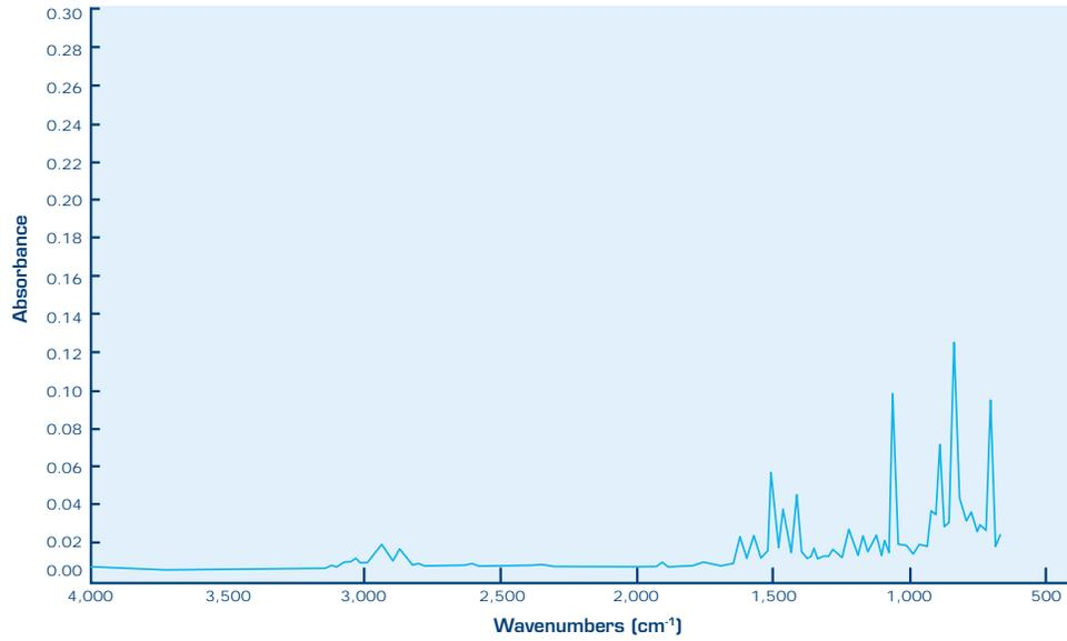
Figure 7. FTIR Absorbance Spectrum of Parylene D
