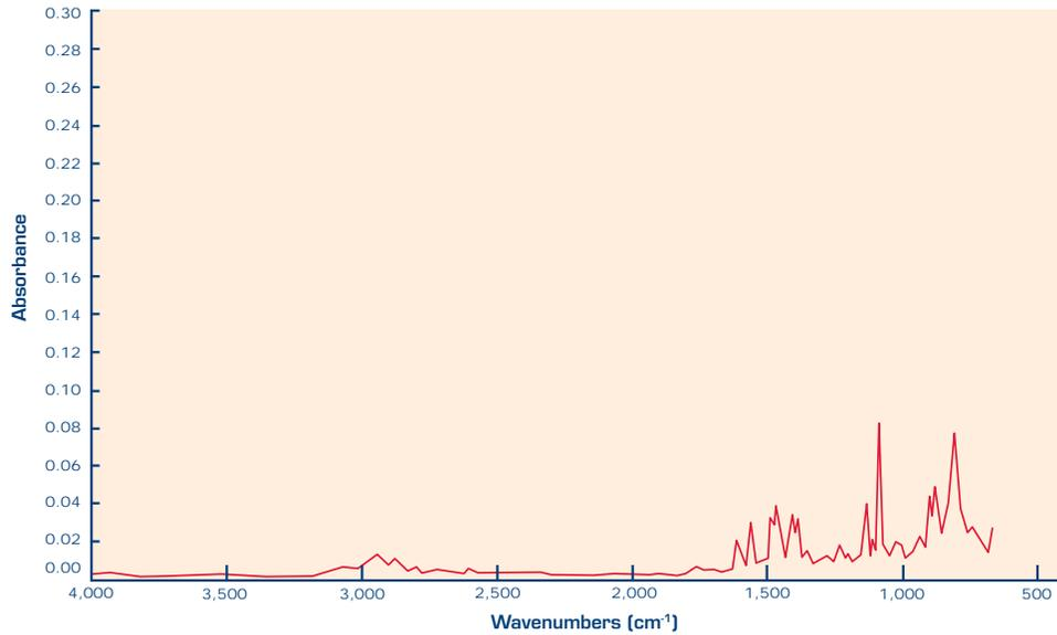
Figure 8. FTIR Absorbance Spectrum of Parylene HT
